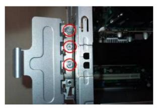
3.3 Press the PCI ear lever (highlighted in red) and pull the leaver outwards a little to release the PCI latch then remove it.
